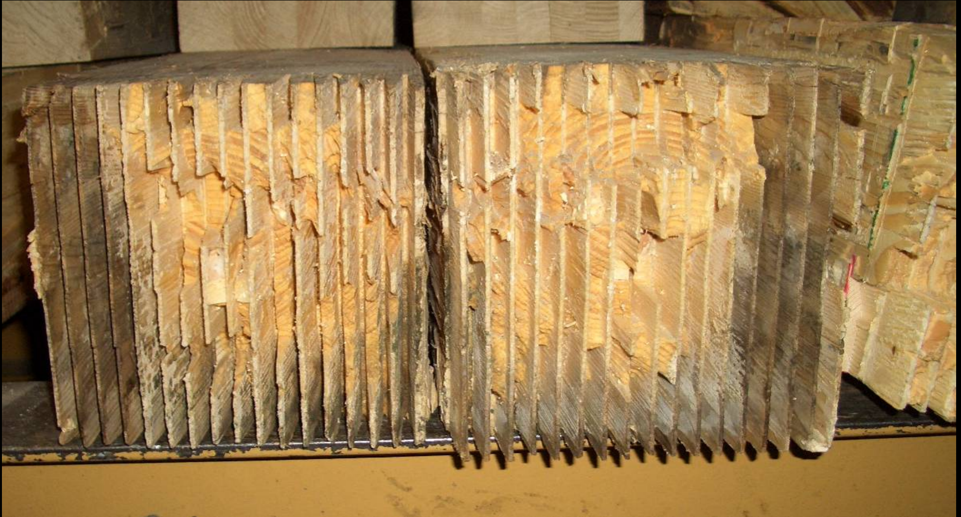
General finger joints – Loss of adhesive effect of UF-glue
